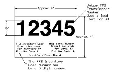
NAMEPLATE: Shall be stainless steel or aluminum with laser etching with contrast lettering and shall be permanently mounted on the tank. Nameplate data shall include as a minimum: transformer weight, impedance, high and low voltage ratings, winding material, KVA rating, date of manufacture, name of supplying manufacturer, wiring schematic, type of insulating fluid, and other data as required by ANSI C57.12.00 standards.
