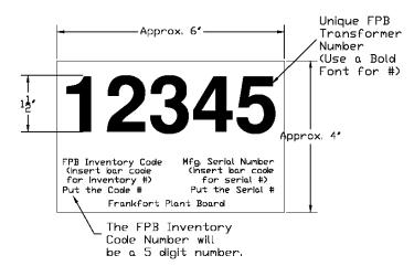
NAMEPLATE: Shall be stainless steel and shall be permanently mounted on the tank or the mounting bracket. Nameplate data shall include as a minimum: transformer weight, impedance, high and low voltage ratings, winding material, KVA rating, date of manufacture, name of supplying manufacturer, wiring schematic, type of insulating fluid, any other data as required by ANSI C57.12.00 standards.
