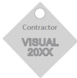
This diamond shaped tag represents that a visual inspection **only** was performed. This tag shows CONTRACTOR's name, identifies that a visual inspection was performed, and the actual year the work is performed.
