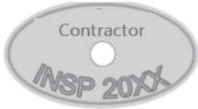
This oval tag is to be used whenever a sound and bore or partial excavate inspection takes place. The tag shows CONTRACTOR's name and the actual year the work is performed.
