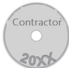
This round tag represents an inspection via a full 18" excavation and treatment with an approved paste. The tag shows CONTRACTOR's name and the actual year the work is performed.
