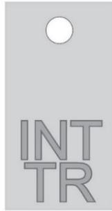
This tag is used whenever internal treatment is injected into a pole. This tag will be used in conjunction with one or more of the above tags depending on the type of inspection performed.
