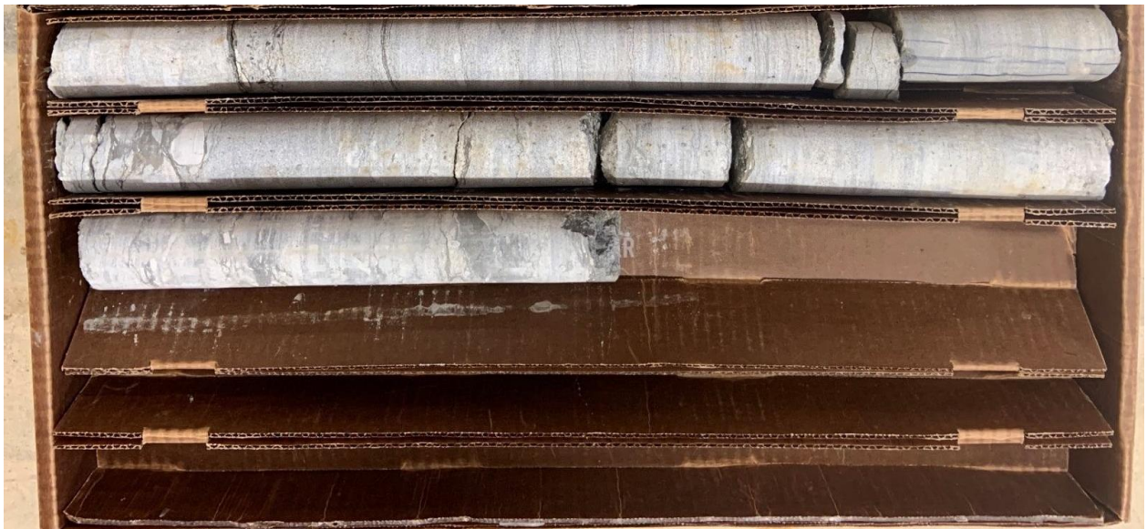
Photo 4. Rock Core at boring B-1 for the depth from 13.5 to 18.5 feet
