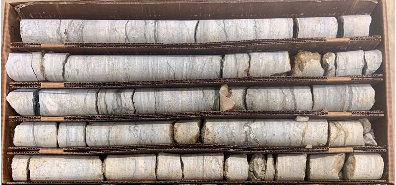
Photo 3. Rock Core at boring B-1 for the depth from 3.5 to 13.5 feet
