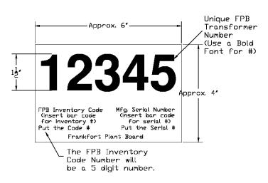
NAMEPLATE: Shall be stainless steel and shall permanently mounted on the tank or the mounting bracket. Nameplate data shall include as a minimum: transformer weight, high and impedance, voltage low ratings. winding material, KVA rating, date of manufacture, name of supplying manufacturer, wiring schematic, type of insulating fluid, any other data as required ANSI C57.12.00 by
