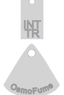
This tag is used whenever internal treatment is injected into a pole. This tag will be used in conjunction with one or more of the above tags depending on the type of inspection performed.
